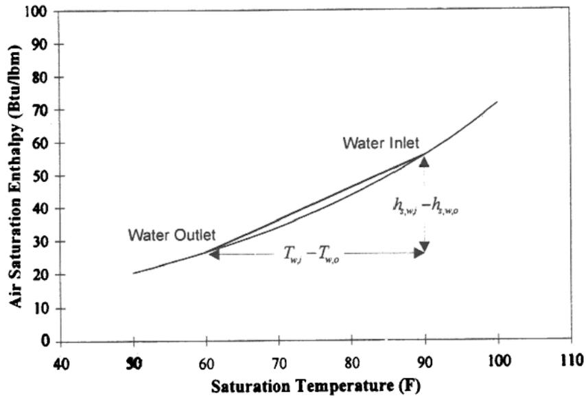
Figure 4.8: Linearization of air saturation enthalpy [58]
