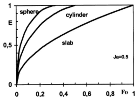
Figure 2.3: Energy released versus time for different geometries [124]
