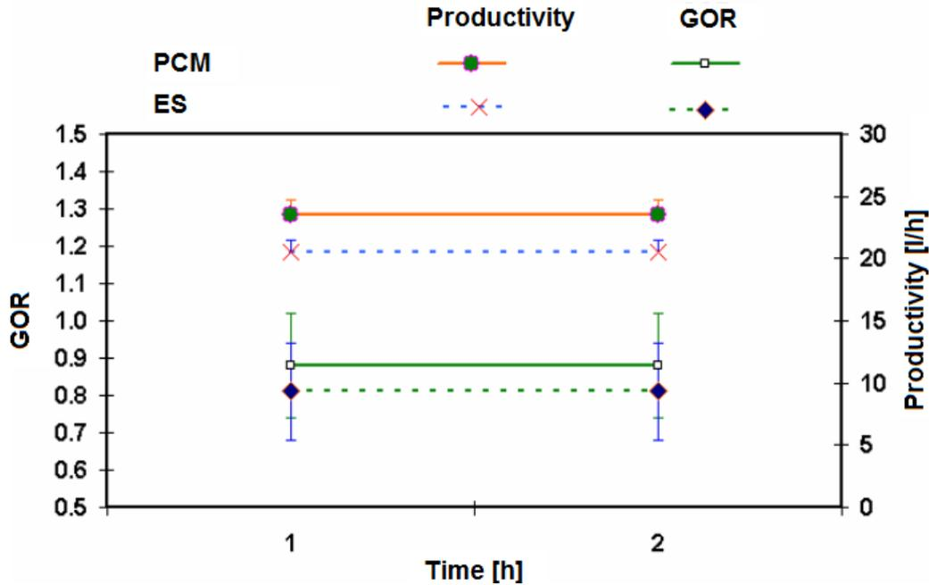
**Figure 5.9: Evolution of productivity and GOR for PCM and Empty balls packing elements**
