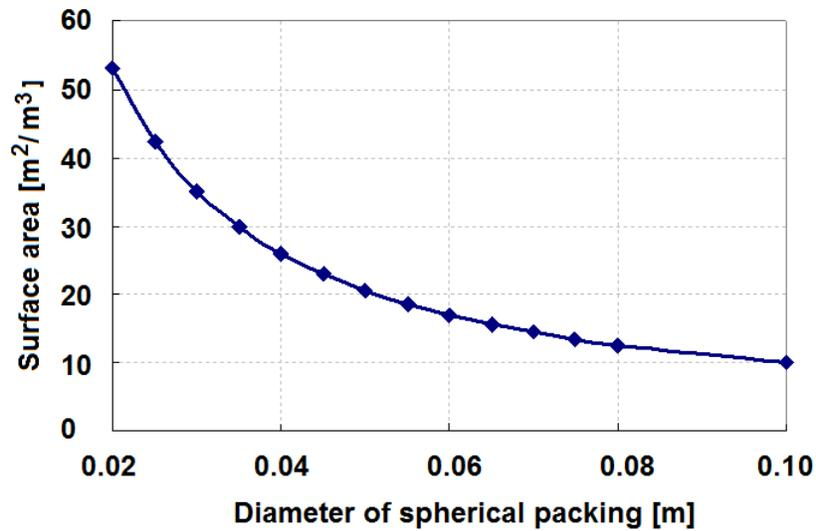
Figure 7.1: Effect of packing size on specific surface area of the packed bed
