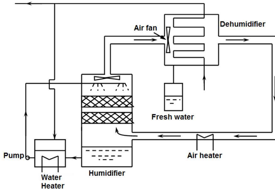
**Figure 2.11: Schematic of HDD system by Abdel-Monem [145]**
