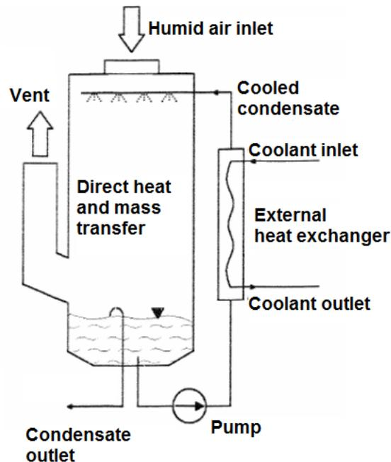
**Figure 2.17: A schematic direct contact spray condensers [148]**
