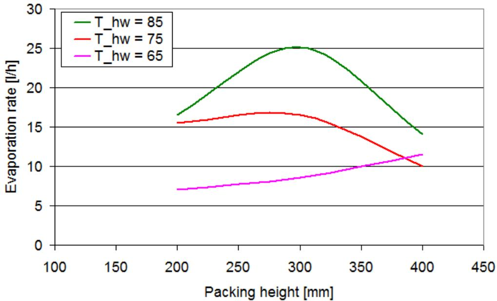
**Figure 2.16: Height versus vapor production for EnviPac filling [128]**
