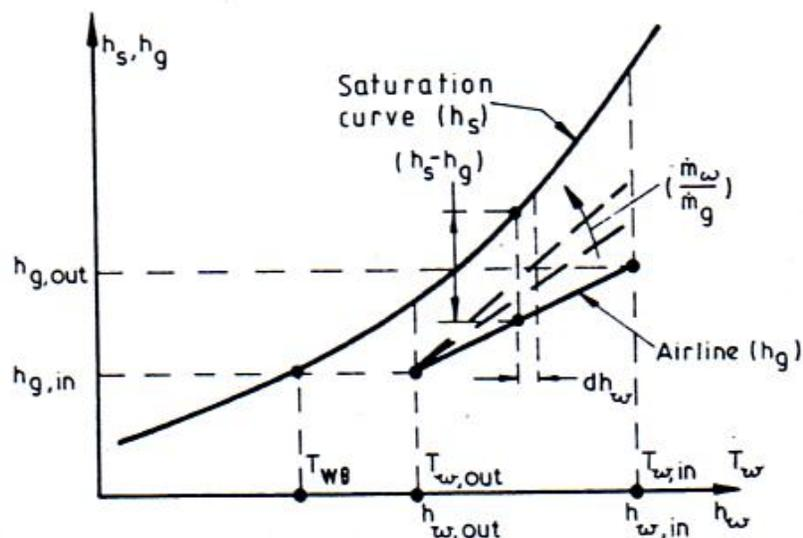
Figure 4.9: Counter current cooling tower operating lines [56]
