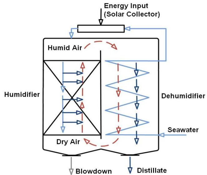
**Figure 1.6: Schematic diagram of a HDH desalination cycle**
