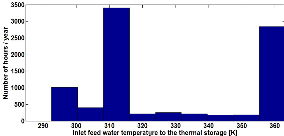
**Figure 8.11: Histogram of hourly variation of inlet water temperature to the PCM-storage over one year for Al-Arish city with 3m<sup>3</sup> thermal storage**
