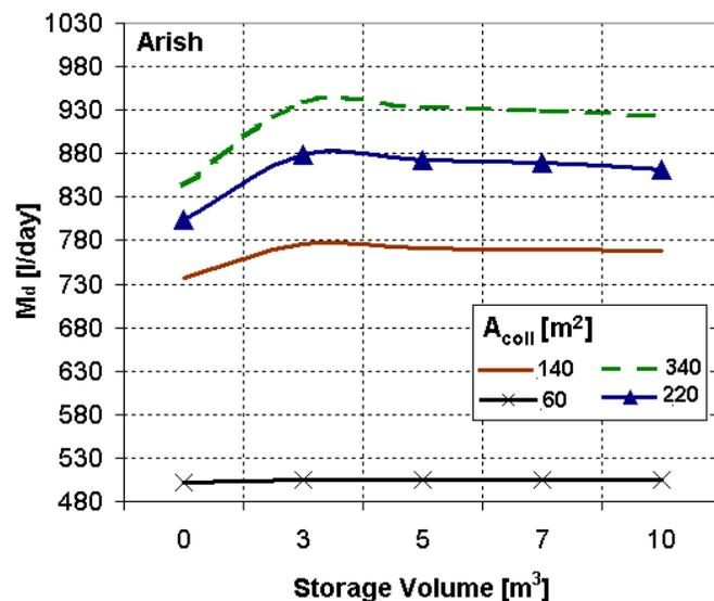
**Figure 8.4: Effect of PCM thermal buffer volume on the average-yearly daily distillate for Al-Arish**
