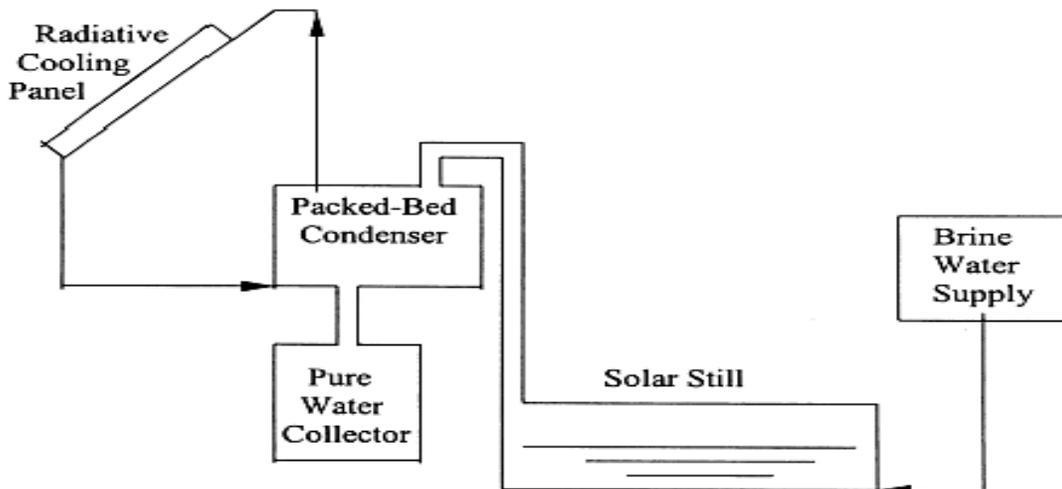
Figure 2.18: Schematics of the radiative cooled solar still [140]
