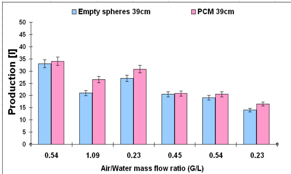
Figure 5.10: Comparative productivity; (Top) 78cm packed height, (Bottom) 39cm packed height
