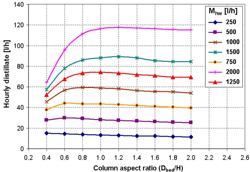
**Figure 7.5: Effect of column aspect ratio on the evaporation rate,  $H=1\text{m}$**
