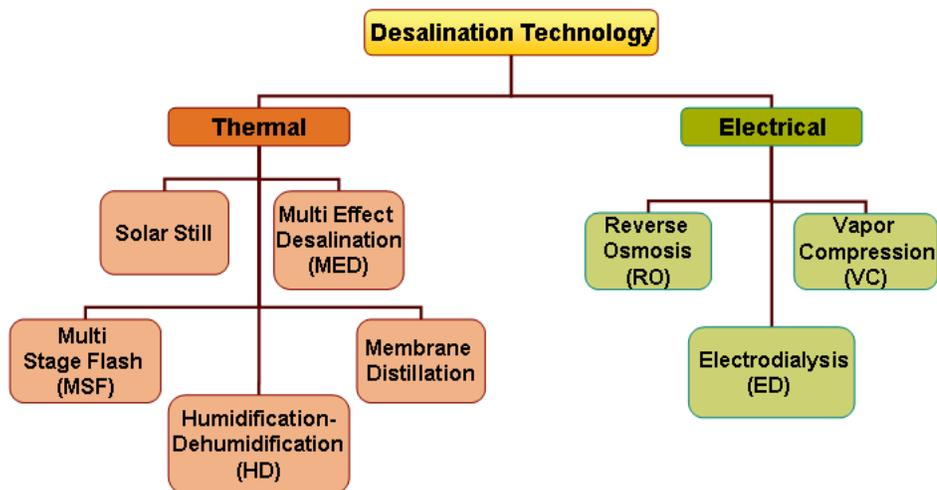
**Figure 1.2: Overview and energy classification of desalination processes**
