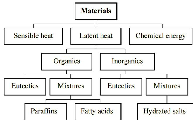
(a) According to type of thermal energy storage media [93]
