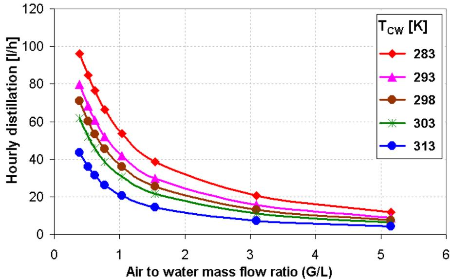
Figure 7.14: Effect of air to water mass flow ratio on the condensation rate
