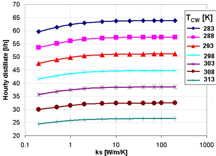
Figure 7.18: Effect of PCM thermal conductivity on condensation rate under different inlet cooling water
