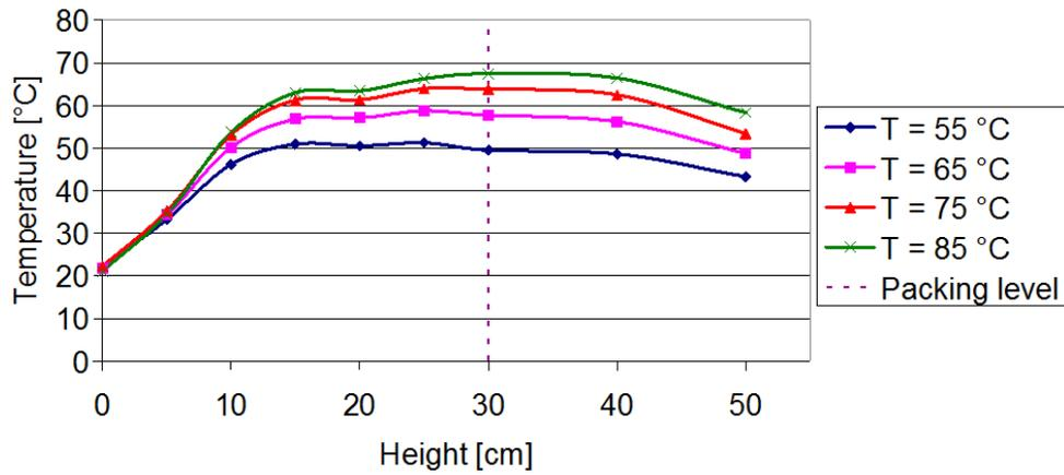
**Figure 2.15: Height versus air temperature for EnviPac [128]**
