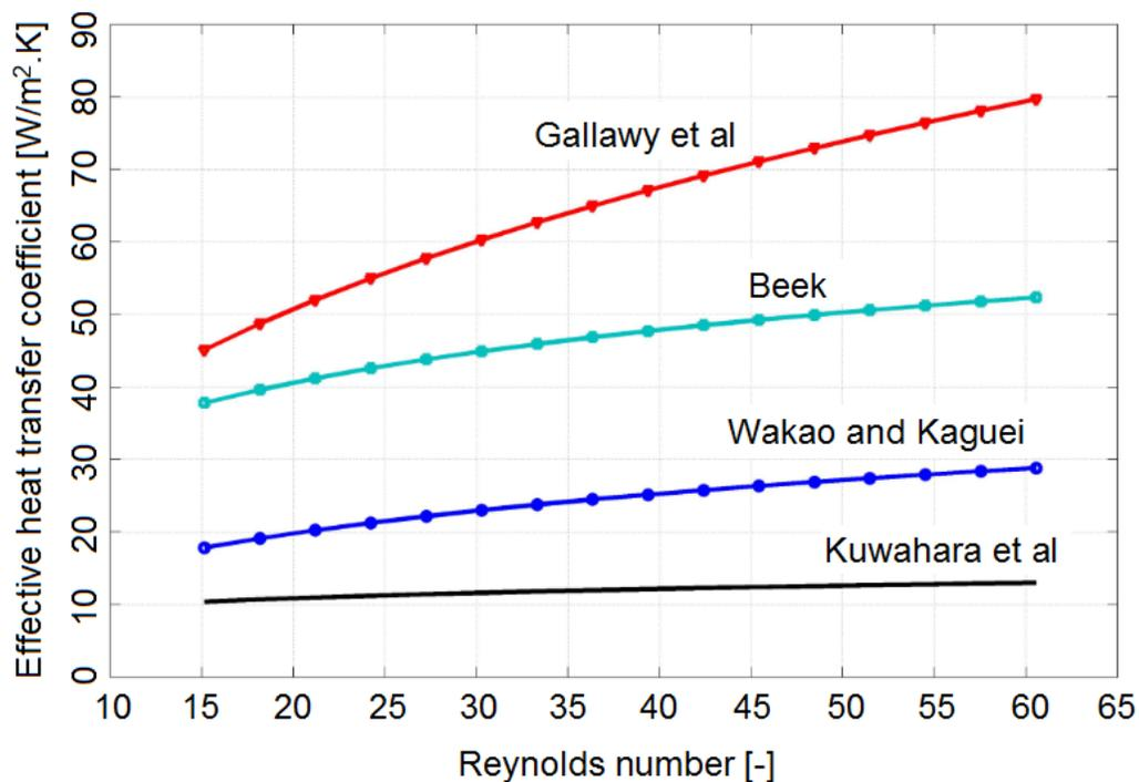
**Figure 4.6: Effective heat transfer coefficients obtained with different Nusselt number correlations.**
