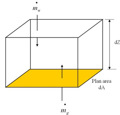
**Figure D.1: Counter flow through an element of the packing region [5]**
