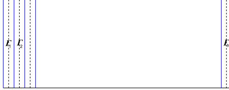
Figure 5.2: Domain decomposition into the inlet boundary domain and the inner domain for the integral computation resulting from the inner products for a discrete case
