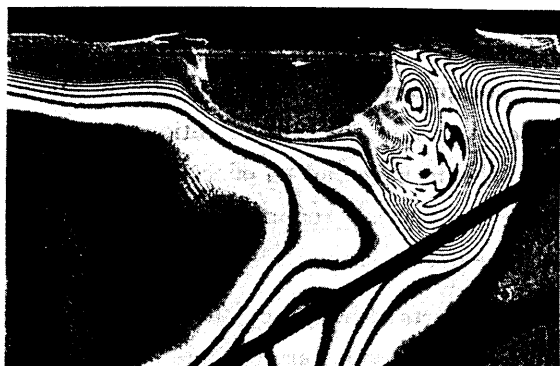
Figure 5: Thermocapillary flow in subcooled R113 observed by holographic interferometry. The bubble is in upside-down position
