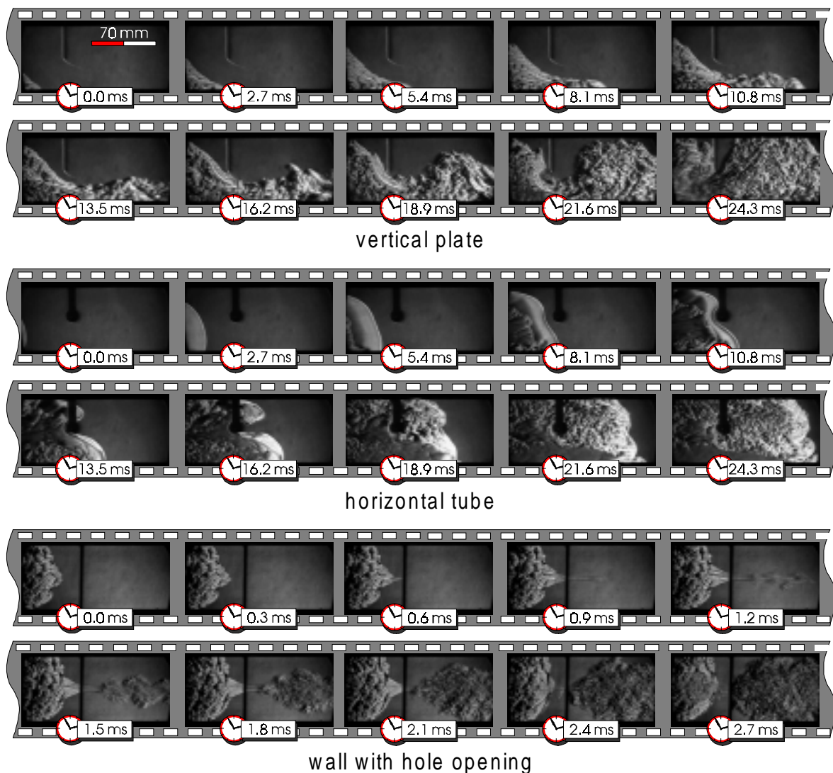
Figure 20: High speed Schlieren video technique, showing the flame acceleration by obstacles during the combustion process of hydrogen in air in a closed tube.
