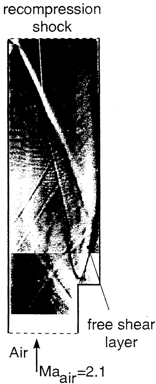
Fig. 1: Flow structure of a supersonic flow over a rearward facing step at Ma_{air} = 2.1
