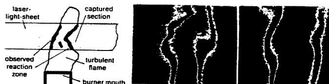
Fig 25: Reaction front of a nonpremixed H_2 -air-flame detected by laser-induced fluorescence
