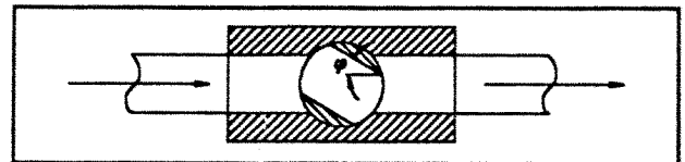
Fig.3 Cut through the ball valve with a closing angle \phi of 30 degree
