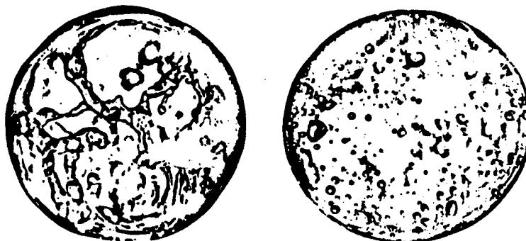
Fig.2: Entrainment and distribution of liquid film in a tube /1/
