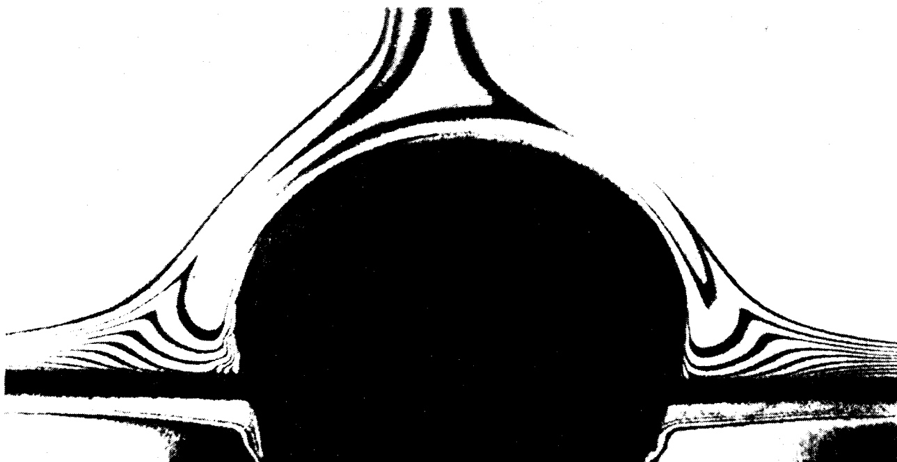
Figure 16.3: Temperature distribution round a "secondary bubble". Water, p = 0.3 bar, \dot{q} = 30 W/cm 2 , subcooling = 2K
