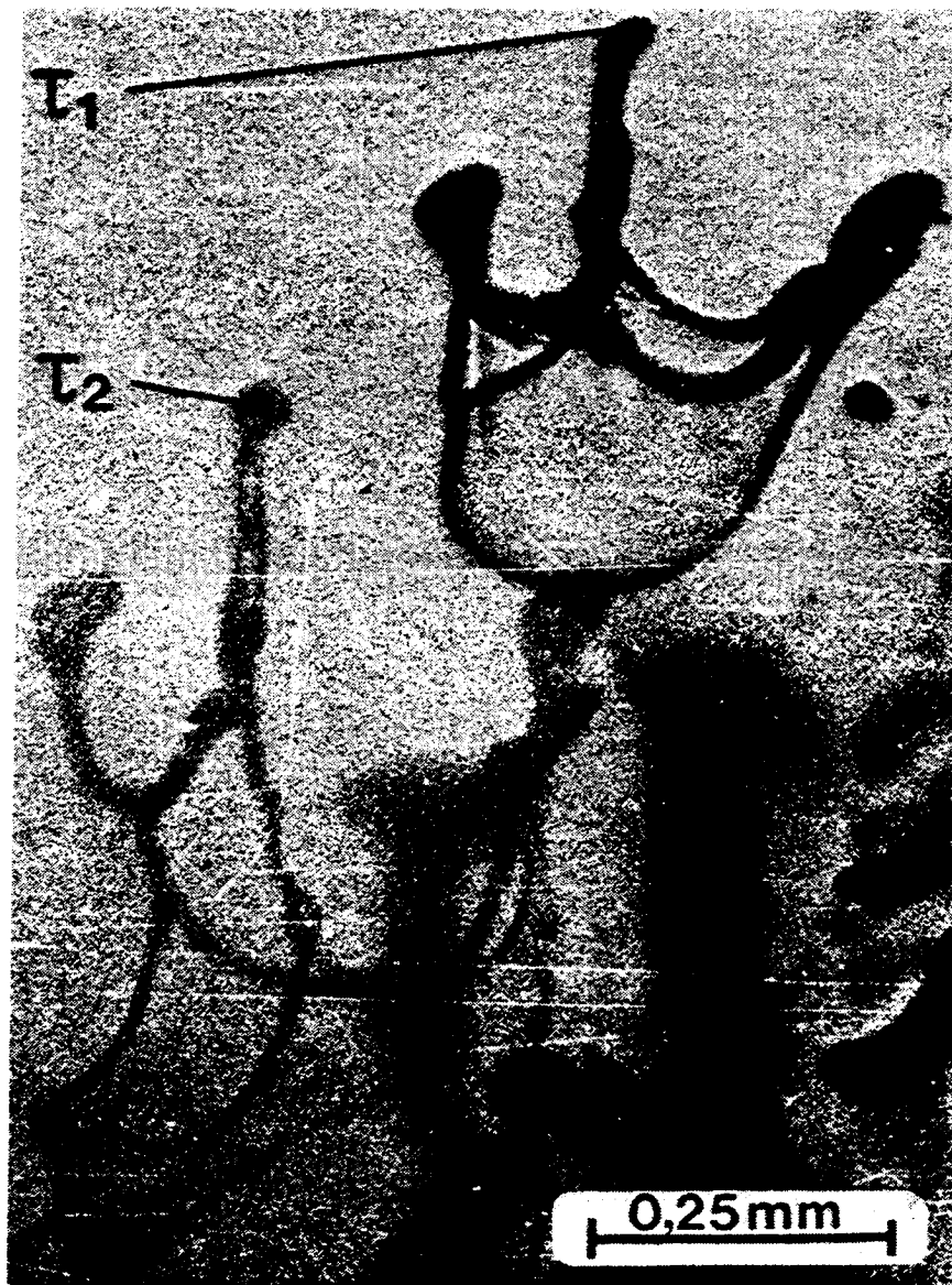
Figure 16.20: Water particle in venture scrubber, double exposure ( \Delta\tau = 10^{-5} s)
