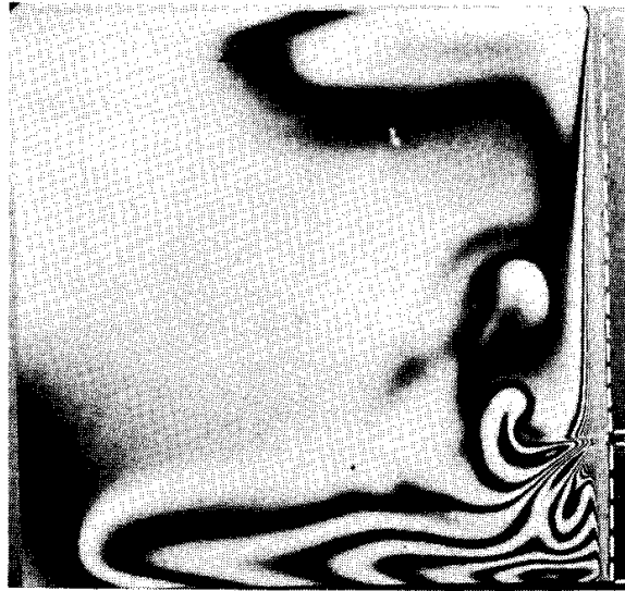
Fig. 10 Interaction between the downward flow on a cold window and the upward flow on a heater.
