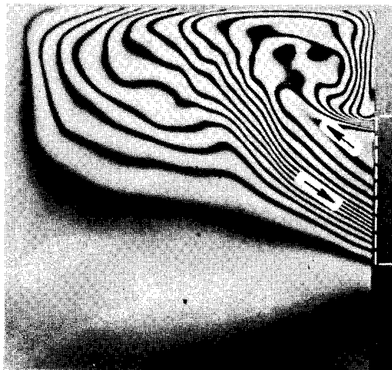
Fig. 11 Air exchange through a window in Summer (outside air warmer)
