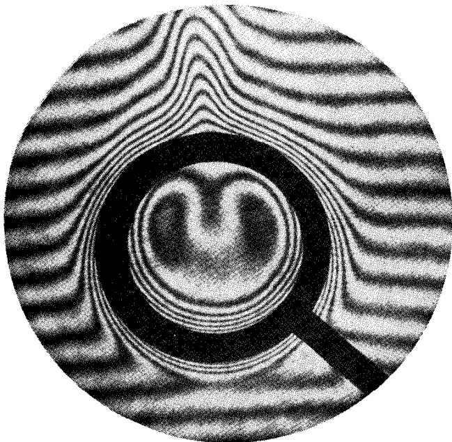
FIG. 7. Temperature field around a horizontal cylinder in air at a temperature 14^{\circ}\text{C} above that of the ambient air.
