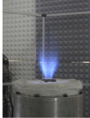
(b) Sound absorbing chamber holding the burner and the probe support frame.
