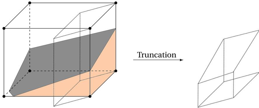
**Figure 3.5:** Principle of unsplit multi-dimensional geometric advection: Reconstructed interface (gray), flux polyhedron (dotted on the left) and advected volume (dotted on the right); Adapted from [135]
