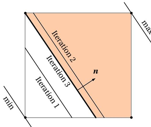
**Figure 3.4:** Principle of iterative interface positioning to fulfill local volume conservation: Two-dimensional example adapted from [220]
