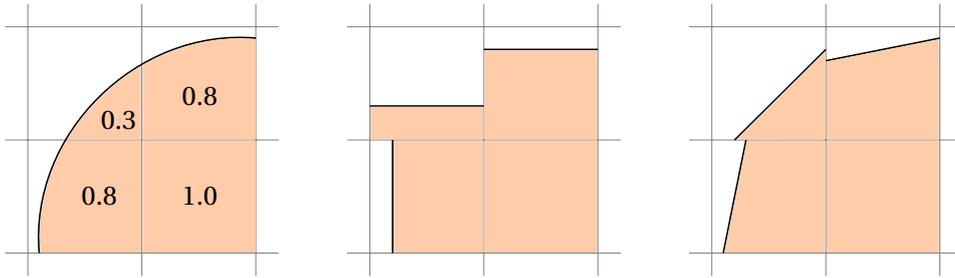
**Figure 3.1:** Exact interface position including discrete volume fraction values  $\alpha$  (left), SLIC-reconstructed interface (center), PLIC-reconstructed interface (right); Two-dimensional example adapted from [220]
