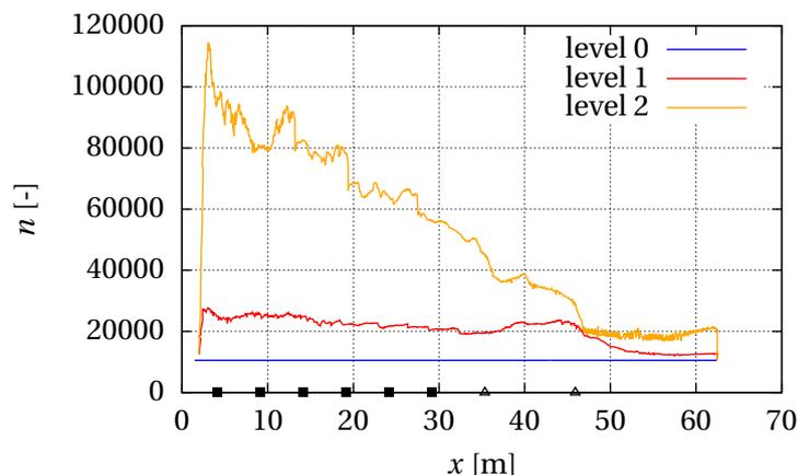
**Figure 4.26:** RUT 22: Overall cell count evolution for different maximum refinement levels
