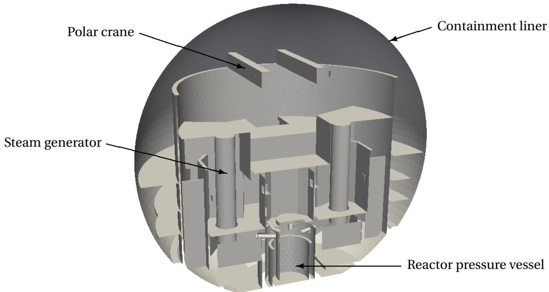
**Figure 5.1:** Sectional view of the Konvoi-type pressurized water reactor model
