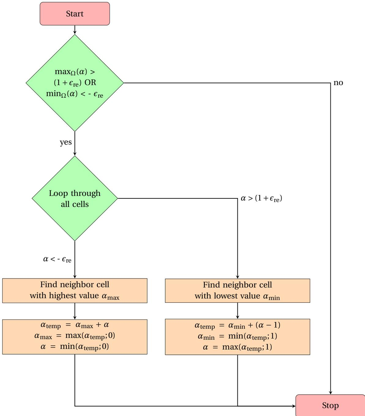
**Figure 3.8:** Schematic of the modified redistribution algorithm
