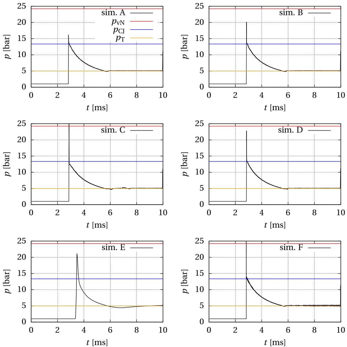
**Figure 3.18:** Temporal pressure profiles (fixed observer) for one-dimensional detonation propagation; Variation of volumetric reaction models and cell size:
