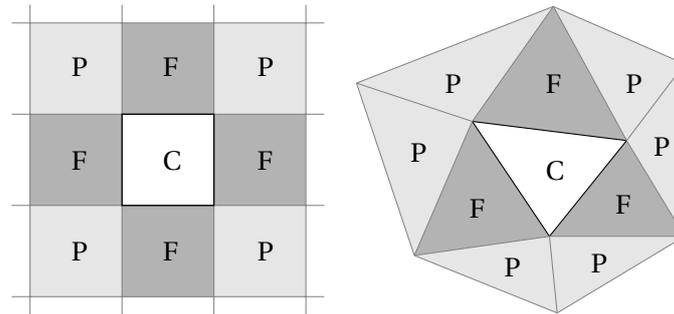
**Figure 3.2:** Two-dimensional stencil of a cell  $C$  with face neighbors  $F$  and point neighbors  $P$ : Structured orthogonal mesh (left) and unstructured triangular mesh (right); Adapted from [135]
