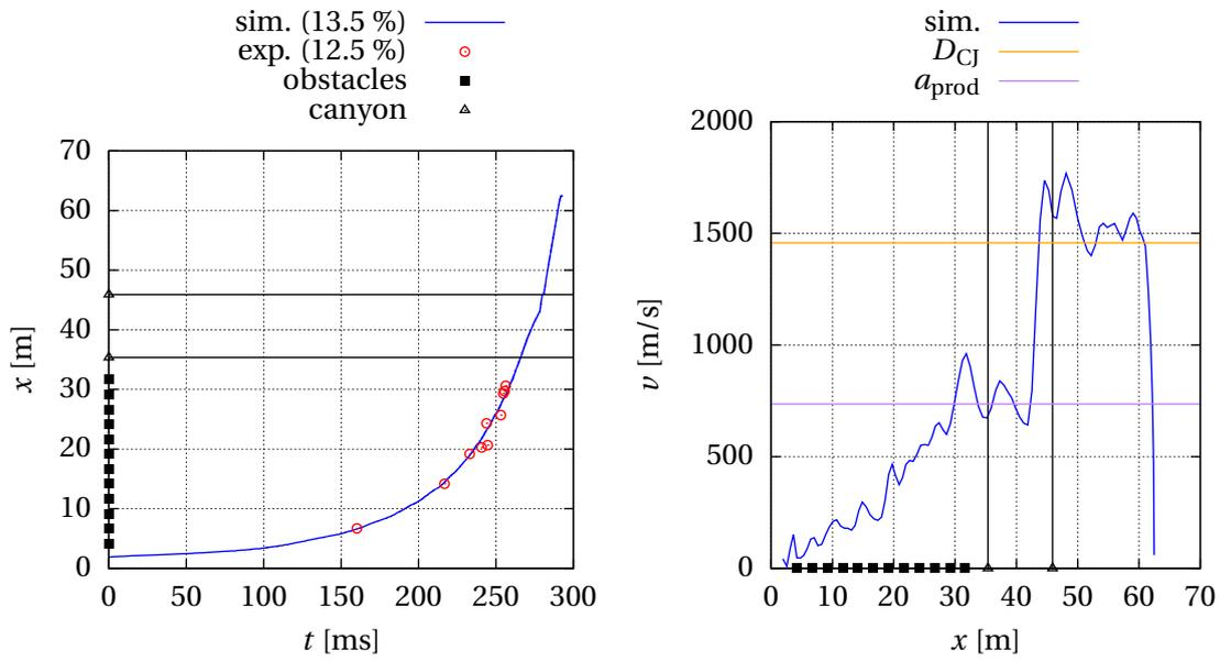
**Figure 4.10:** RUT 16 with increased hydrogen content of 13.5 %: Flame-tip acceleration
