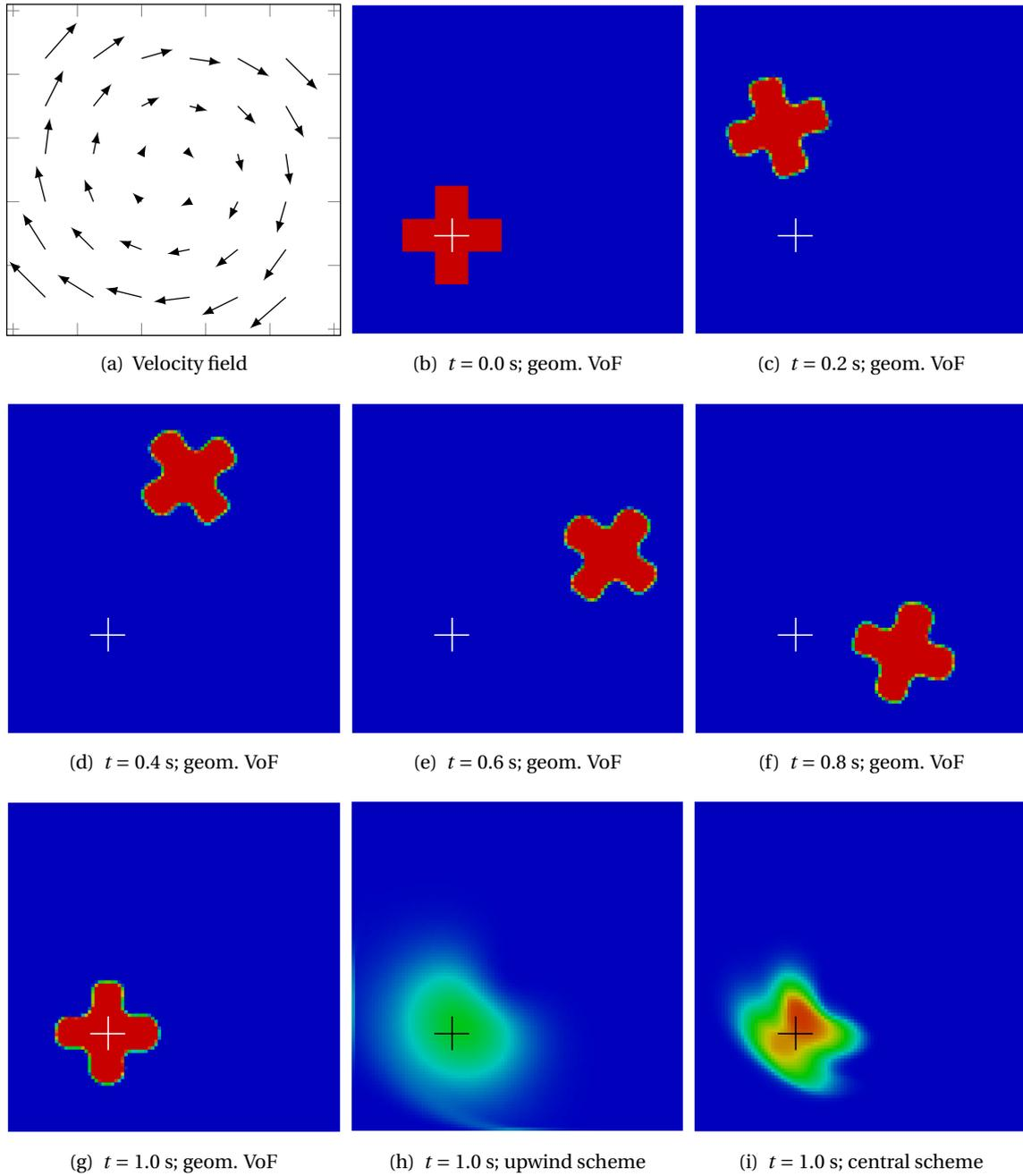
**Figure 3.9:** Non-reactive rotating cross example: Velocity field including magnitude-scaled arrows; Volume fraction at different points in time and by using different discretization schemes; Rainbow color scale (appendix A) from  $\alpha = 0$  to  $\alpha = 1$
