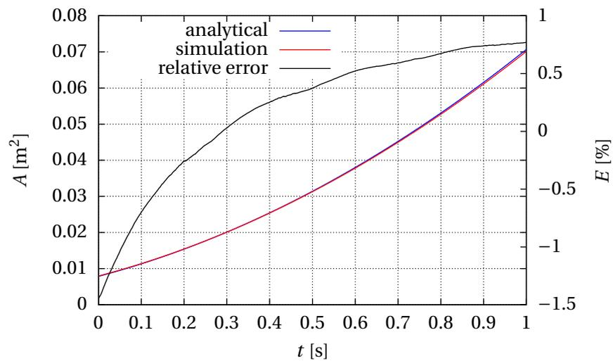
**Figure 3.12:** Rotating reactive circle example: Temporal evolution of circle area  $A$  and relative error  $E$
