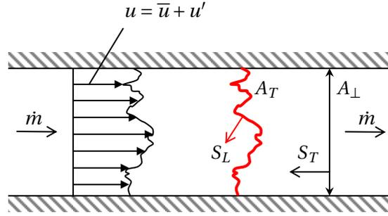
**Figure 3.15:** Topological interpretation of the turbulent burning velocity; Turbulent flame colored red; Adapted from [206]
