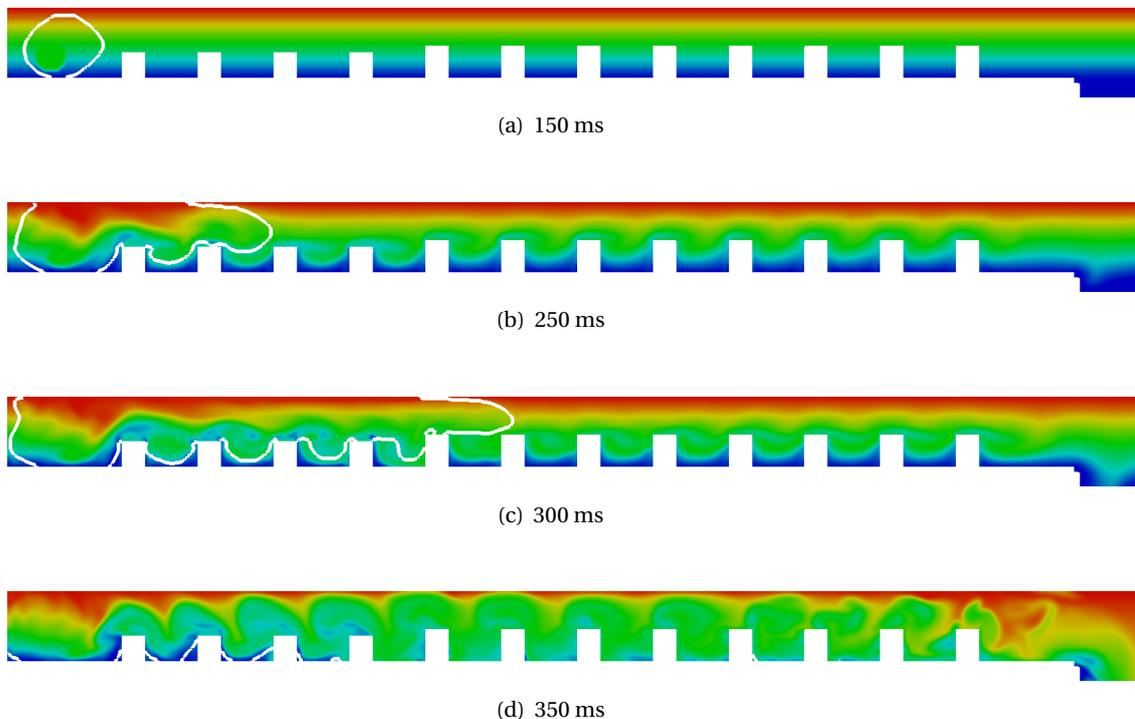
**Figure 4.17:** RUT 'inhomogeneous': Hydrogen mixture fraction at four points in time after ignition; Cutting plane located on the center line of the channel; Rainbow color scale (appendix A) from 10.5 % to 15.5 %
