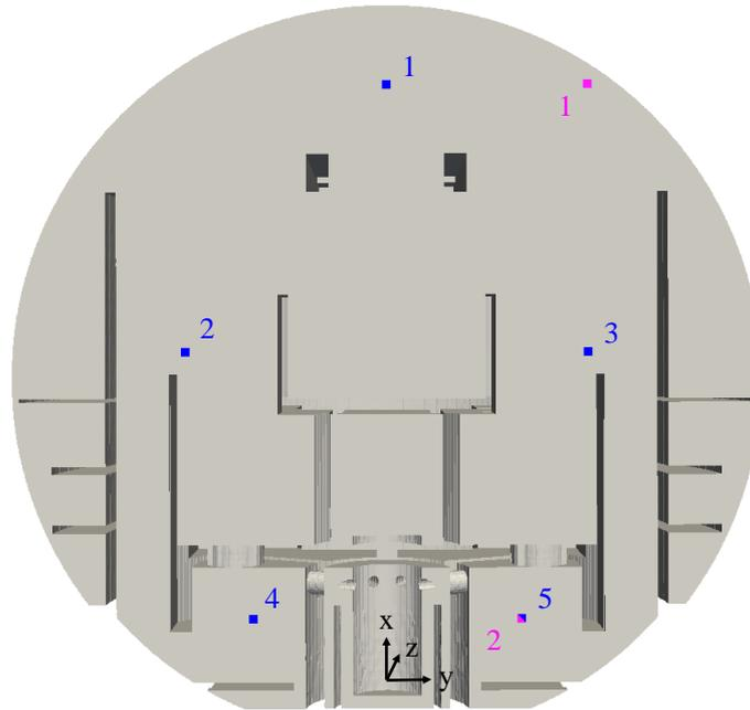
**Figure 5.2:** Ignition (purple) and pressure probe locations (blue)
