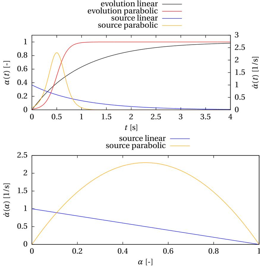
**Figure 3.17:** Evolution of  $\alpha$  and corresponding source term profiles  $\dot{\alpha}$  for both volumetric reaction models in time space  $t$  (top) and reaction progress space  $\alpha$  (bottom)
