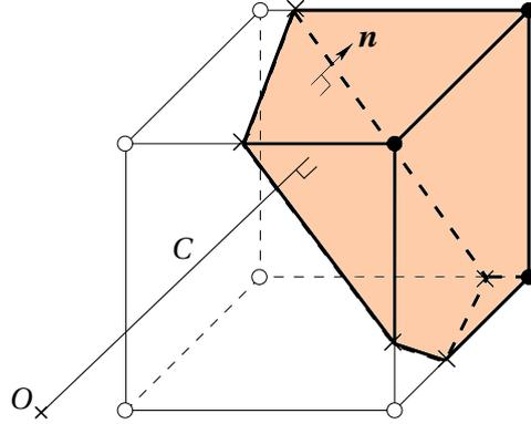
**Figure 3.3:** Truncation of a general polyhedron (vertices  $\bullet$  and  $\circ$ ) by an interface of orientation  $\mathbf{n}$ ; Points of positive signed distance ( $\bullet$ ) and intersection points ( $\times$ ) form the truncated polyhedron (thick lines);  $C$  denotes the interface offset to the origin  $O$ ; Adapted from [170]
