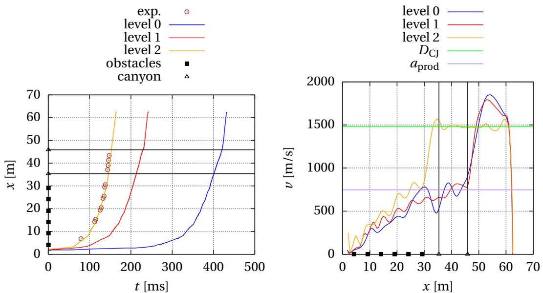
**Figure 4.24:** RUT 22: Flame-tip acceleration for different maximum refinement levels
