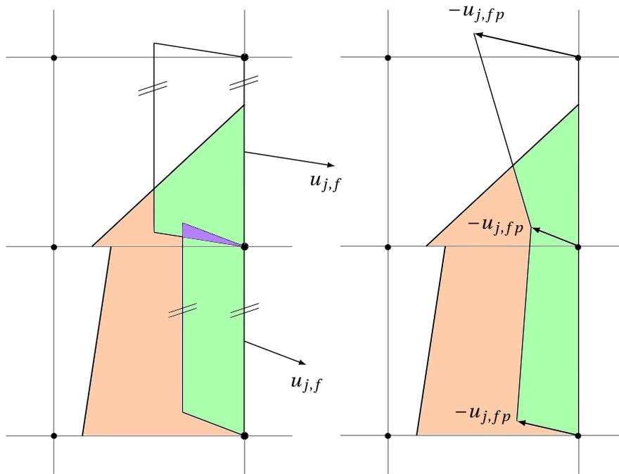
**Figure 3.6:** Advection step mechanism in two dimensions: Based on flux polyhedron construction by face velocities (left) and based on flux polyhedron construction by unique point velocities (right); Different color levels distinguish empty part of cell (white), occupied but not advected part of cell (orange), advected volume (green) and erroneously twice fluxed region (purple); Adapted from [171]
