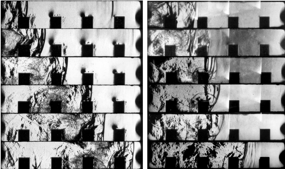
**Figure 2.9:** Shadowgraphy images of the miniRUT facility: Explosion propagation in the obstructed channel without (24 % of hydrogen in air) and with (29.6 % of hydrogen in air) obstacle-induced DDT; Reproduced from [66]
