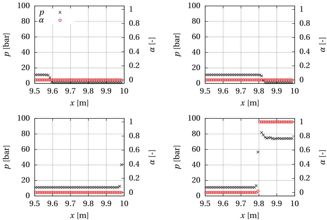
**Figure 3.19:** Temporal evolution of DDT by shock reflection in one dimension: Spatial profiles of pressure  $p$  and reaction progress  $\alpha$ ; Time difference between snapshots is 0.2 ms
