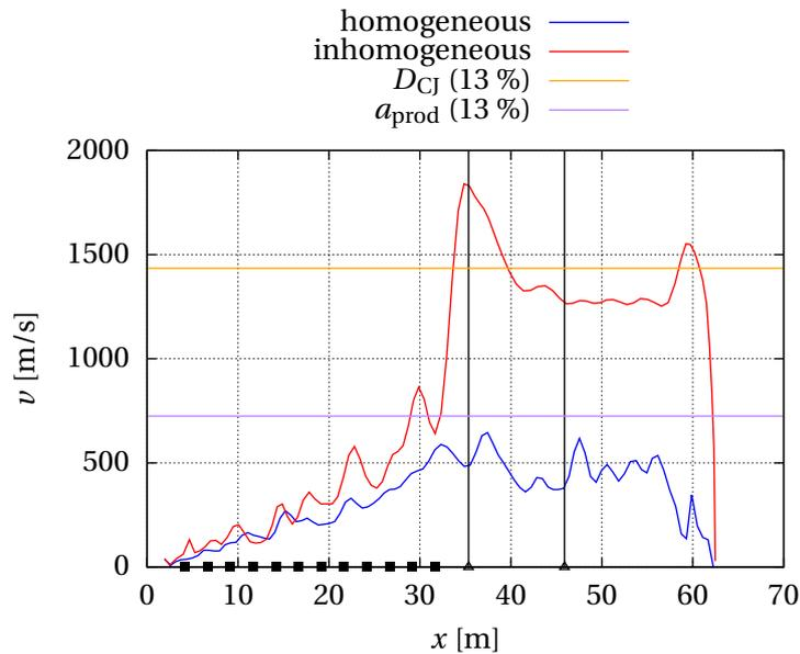
**Figure 4.18:** RUT 'inhomogeneous': Flame-tip acceleration
