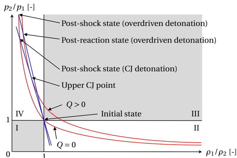
**Figure 2.11:** CJ and overdriven detonation in the Rankine-Hugoniot diagram: Hugoniot curves colored red, Rayleigh lines colored blue
