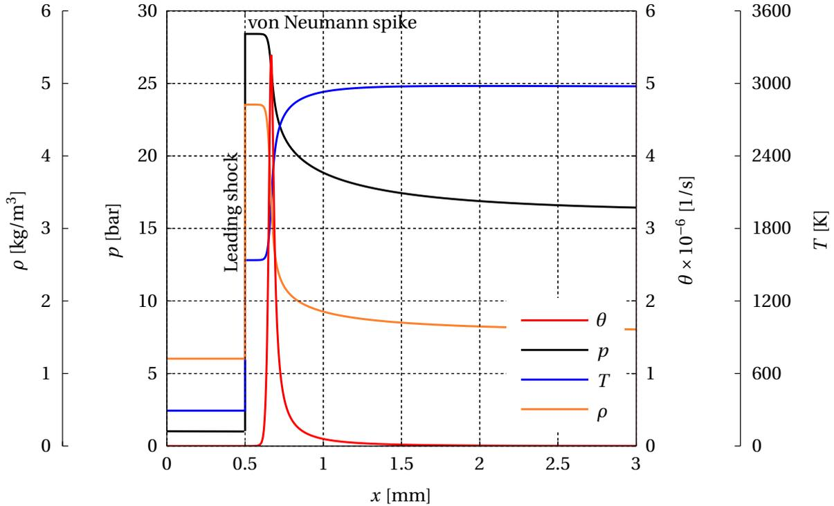
**Figure 2.12:** Internal structure of a CJ detonation according to one-dimensional ZND theory: Spatial profiles of thermicity  $\theta$  (a measure of heat release), pressure  $p$ , temperature  $T$  and density  $\rho$  for a stoichiometric hydrogen-air mixture at ambient initial conditions; Adapted from [122]
