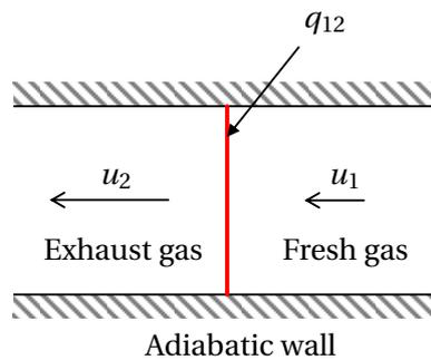
**Figure 2.1:** Schematic of the one-dimensional reaction front model: Reactive discontinuity colored red; Adapted from [17]
