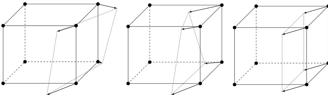
**Figure 3.7:** Flux polyhedron examples resulting from different construction techniques: Non-convex body created from point velocities (left), convex body with non-planar faces created from point velocities (center) and convex body with planar faces created from face velocities (right); Reproduced from [135]
