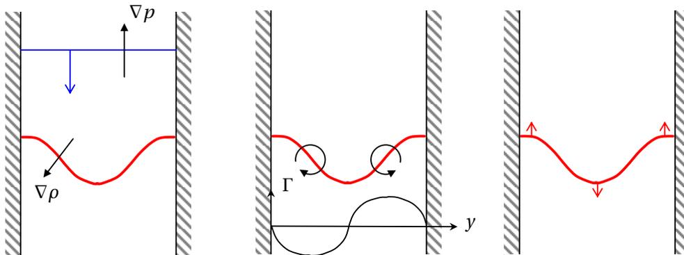
**Figure 2.8:** Schematic of the Richtmyer-Meshkov instability: Flame colored red and incident shock colored blue; Adapted from [45]
