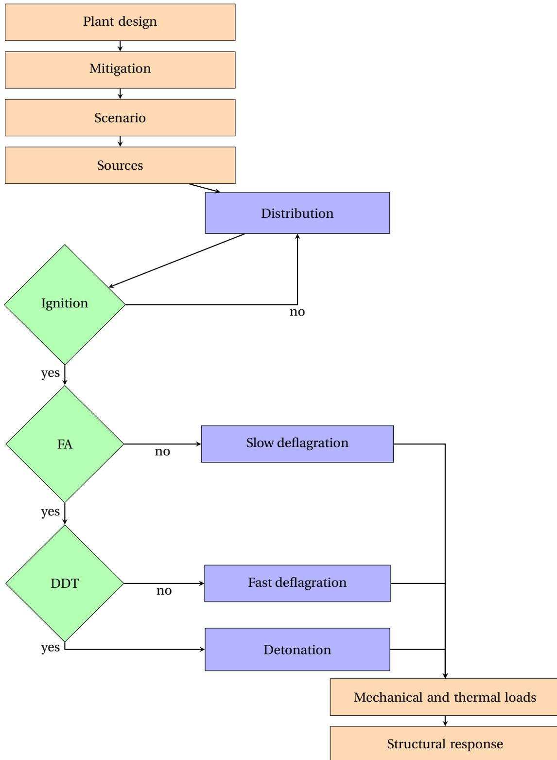
Figure 1.1: Nuclear safety analysis chain according to [39]
