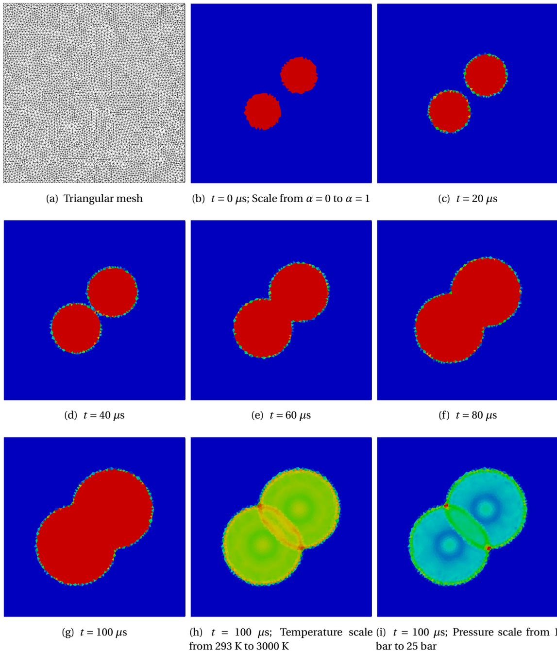
**Figure 3.13:** Merging detonation kernels example: Unstructured mesh, volume fraction, temperature and pressure at different points in time; Rainbow color scale according to appendix A
