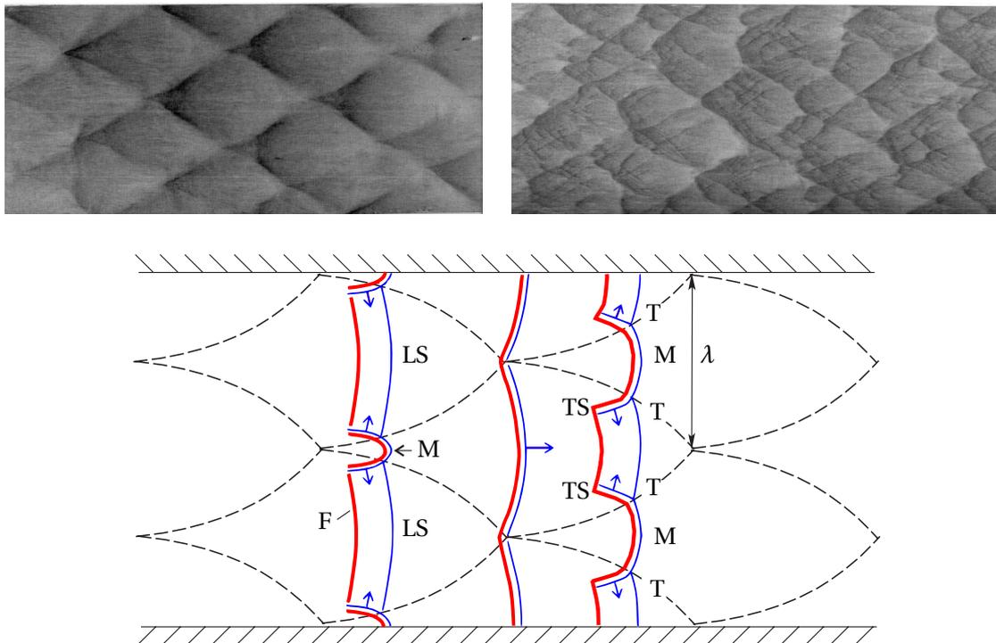
**Figure 2.10:** Multi-dimensional cellular detonation structure: Regular (top left) and irregular (top right) experimental soot print reproduced from [11]; Schematic (bottom) adapted from [74]; Flame colored red and shocks colored blue
