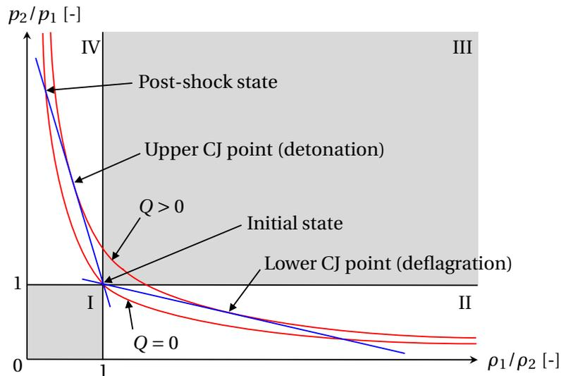
**Figure 2.2:** Rankine-Hugoniot diagram: Hugoniot curves colored red, Rayleigh lines colored blue; Adapted from [157]
