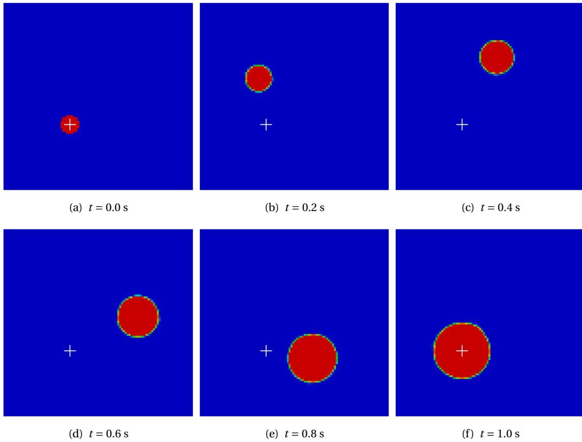
**Figure 3.11:** Reactive rotating circle example: Volume fraction at different points in time; Rainbow color scale (appendix A) from  $\alpha = 0$  to  $\alpha = 1$
