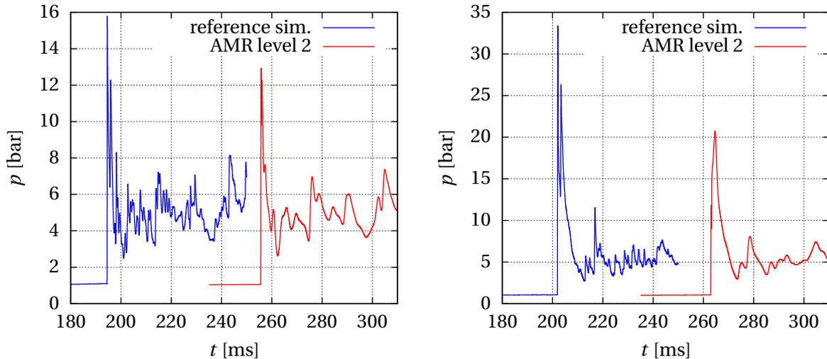
**Figure 4.25:** RUT 22: Transient pressure recordings at sensor 7 (canyon entry, left picture) and sensor 6 (canyon end wall, right picture)
