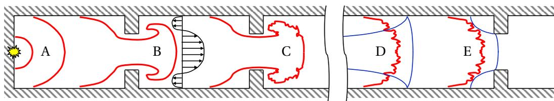
**Figure 2.5:** Phenomenology of FA in obstructed facilities: Flame colored red and shocks colored blue
