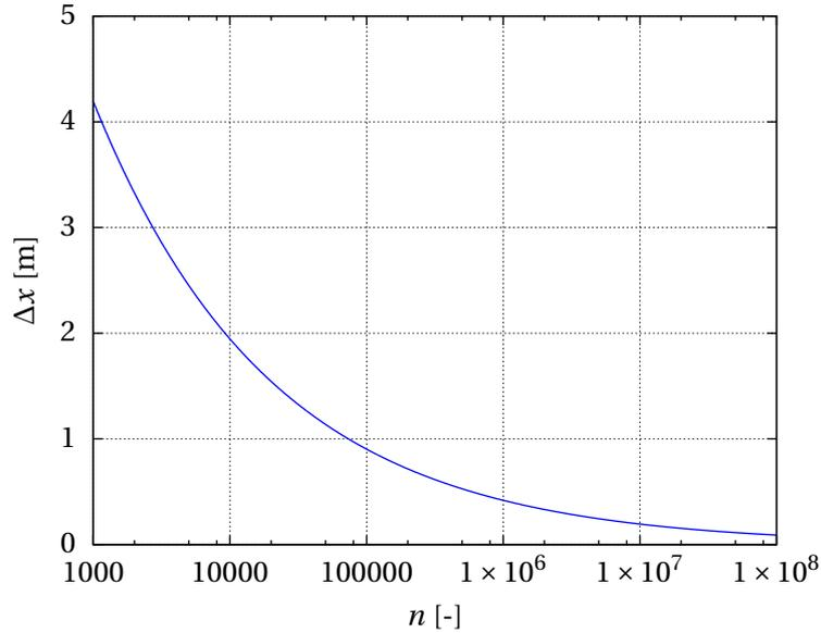
**Figure 1.2:** Dependency of the characteristic cell size  $\Delta x$  on the number of cells  $n$  for a spherical volume of radius  $R = 26$  m
