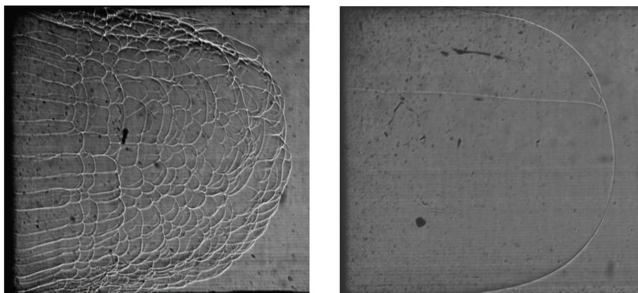
**Figure 2.6:** Shadowgraphy images of unstable (11.5 % of hydrogen in air,  $Le < 1$ ) and stable (29.4 % of hydrogen in air,  $Le \approx 1$ ) early flame propagation in the GraVent facility; Reproduced from [123]
