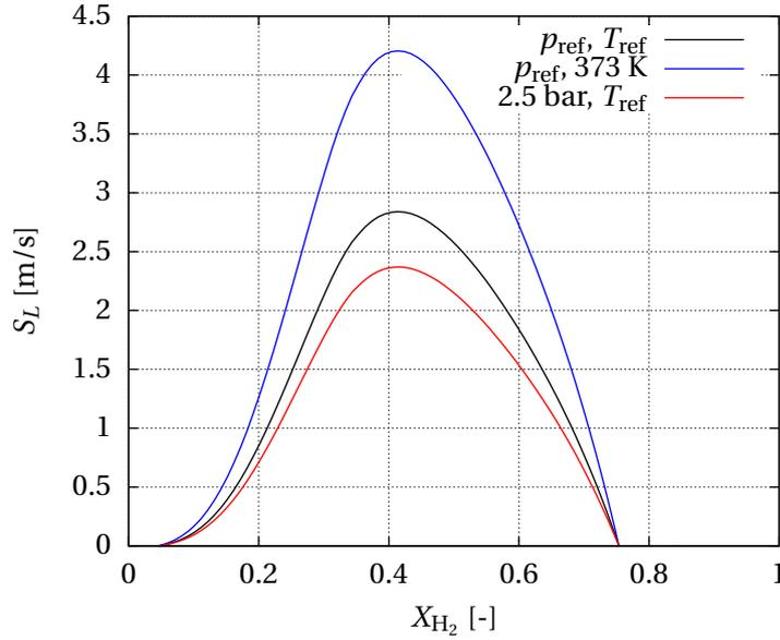
**Figure 3.14:** Laminar burning velocity  $S_L$  depending on mixture composition, temperature and pressure of the unburned gas
