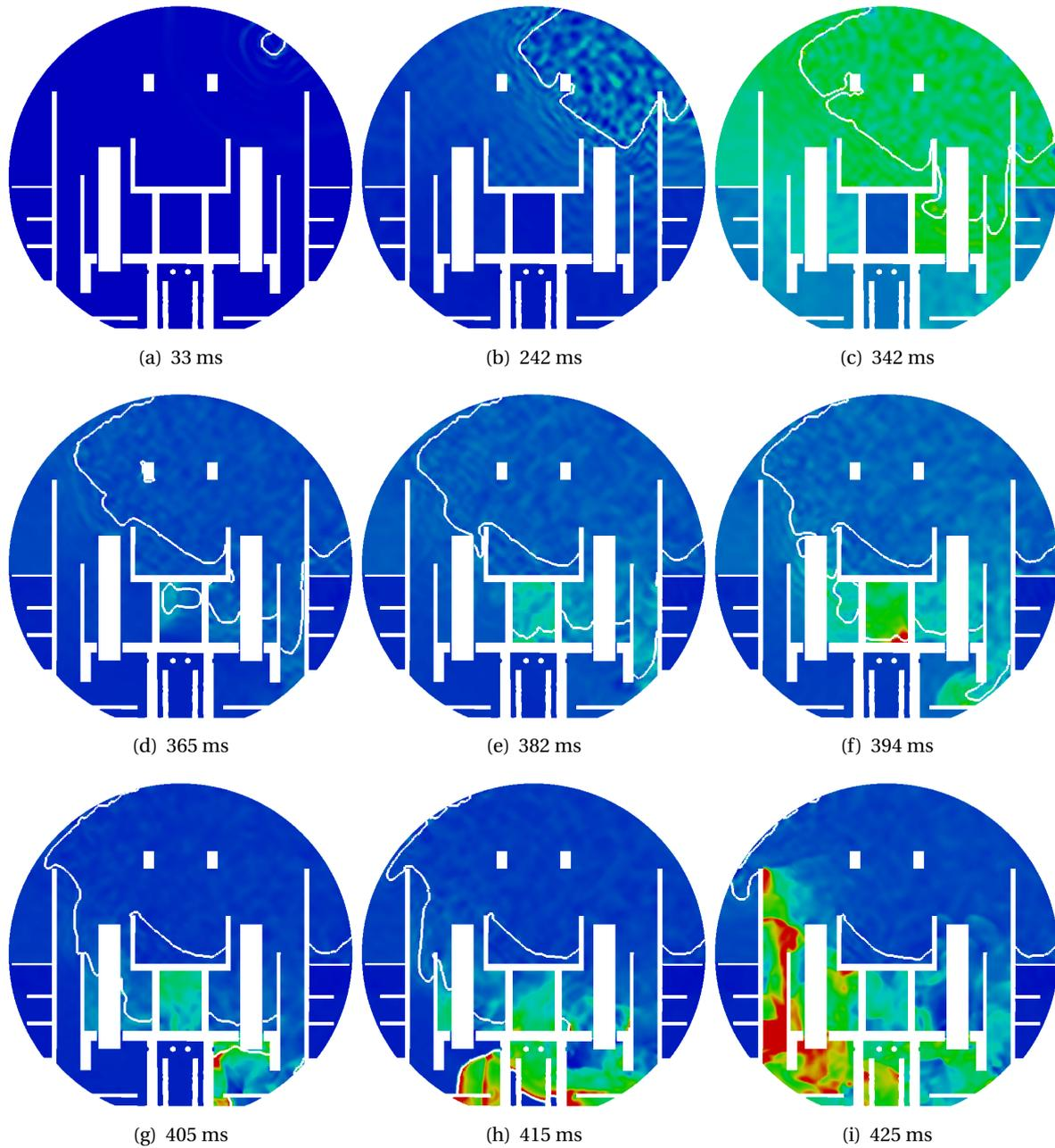
**Figure 5.6:** Pressure field including flame contour;  $\hat{X}_{H_2} = 15\%$ ,  $\Delta X_{H_2} = 0\%$  (homogeneous); Rainbow color scale according to appendix A: First row from 2.5 to 5 bar, second row from 2.5 to 15 bar, third row from 2.5 to 30 bar
