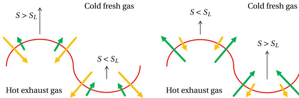
**Figure 2.7:** Schematic of thermal-diffusive instability: Unstable situation on the left ( $Le < 1$ ), stable situation ( $Le > 1$ ) on the right; Flame colored red, heat flux colored green and species flux colored orange; Adapted from [207]
