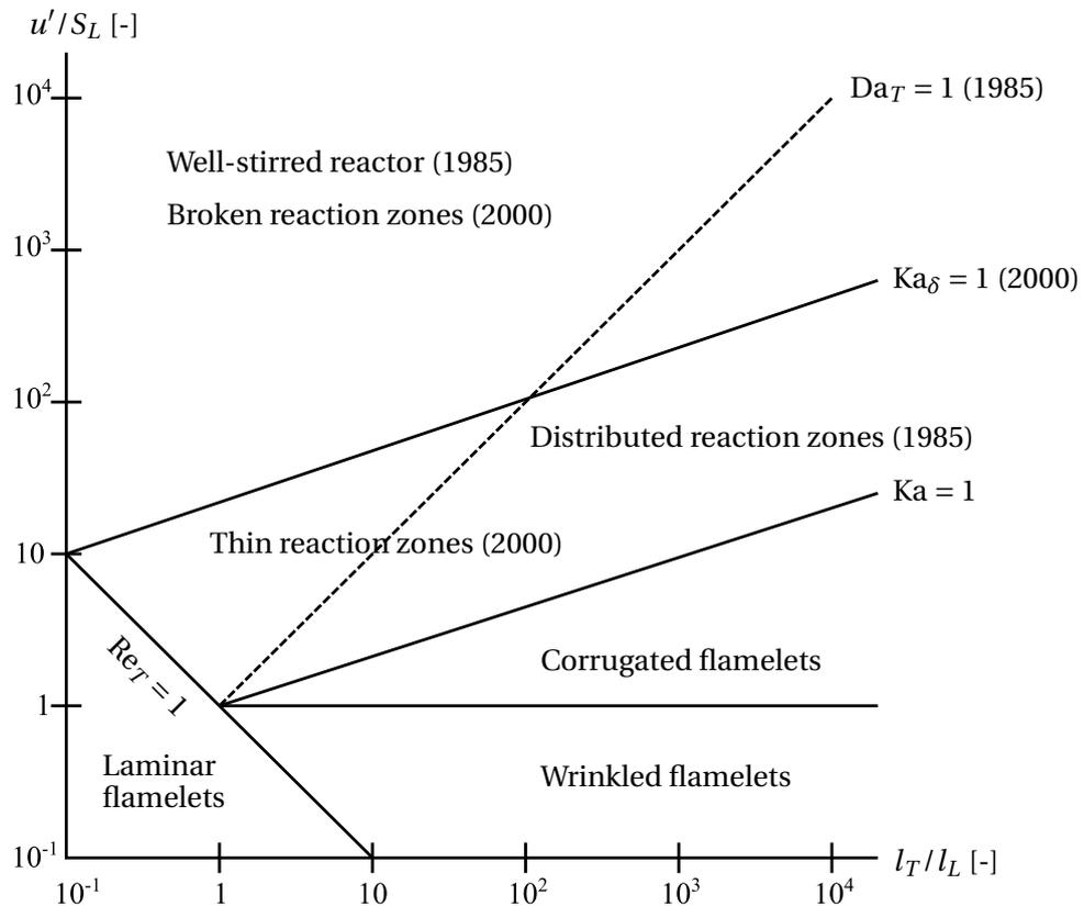
**Figure 2.3:** Regime diagram of turbulent premixed combustion: Versions of Borghi (1985) [32, 33] and Peters (2000) [206] combined
