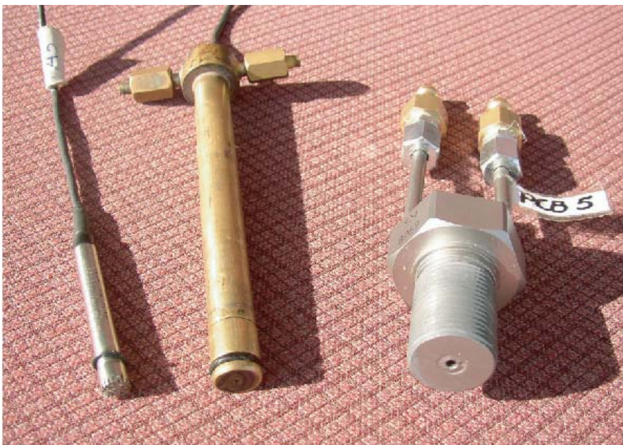
Fig. 4.1: 1/4" condenser microphone (left) with cooling adapter (centre) and PCB piezo-transducer (right).
