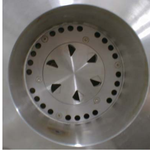
Fig. 3.4: Siren outlet: The excited air flow leaves the siren through the double-sine shaped orifices in the centre, while the bypassed air is injected through the holes in the outer annulus.
