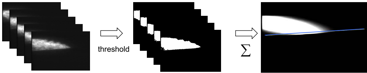
Figure 4.5: Derivation of mean flame position by image interpolation.
