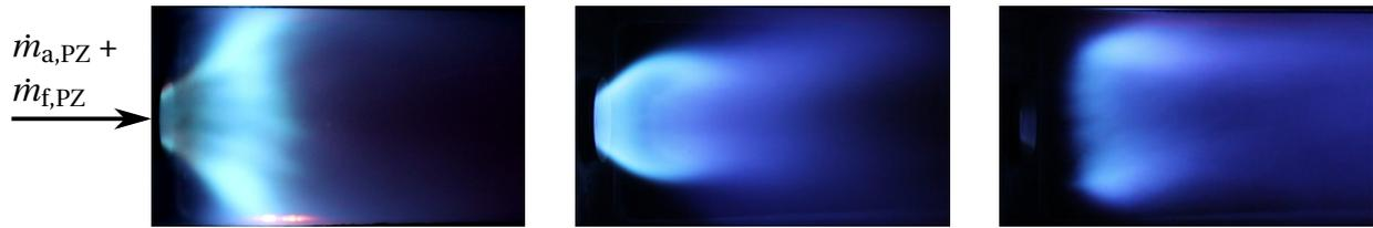
**Figure 5.3:** Flame shapes in the primary zone for an air preheating temperature of  $T_{a,PZ} = 473\text{ K}$  and a thermal power of  $\dot{Q}_{th} = 53.2\text{ kW}$ . Conical flame (left), constricted flame (middle) and lifted flame (right).
