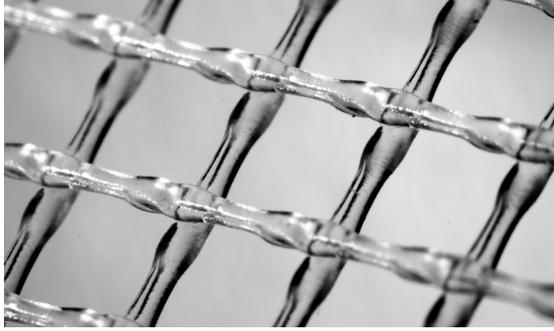
(a) Microscopy image of spacer;  $L_1 = L_2 = 2$  mm,  $\beta = 90^\circ$ .
