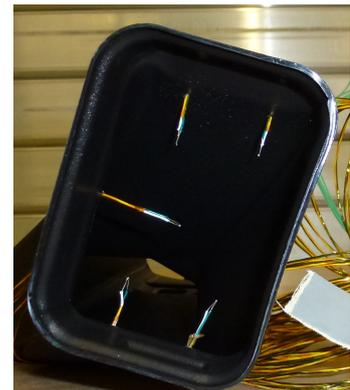
(b) Thermocouples at the inlet of the ventilation duct
