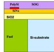
A 2D-axisymmetrical model of the micro-thruster unit. (Oberwolfach Benchmark collection)
