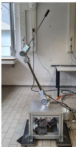
Fig. 1: Experimental robot with rigid and flexible links
