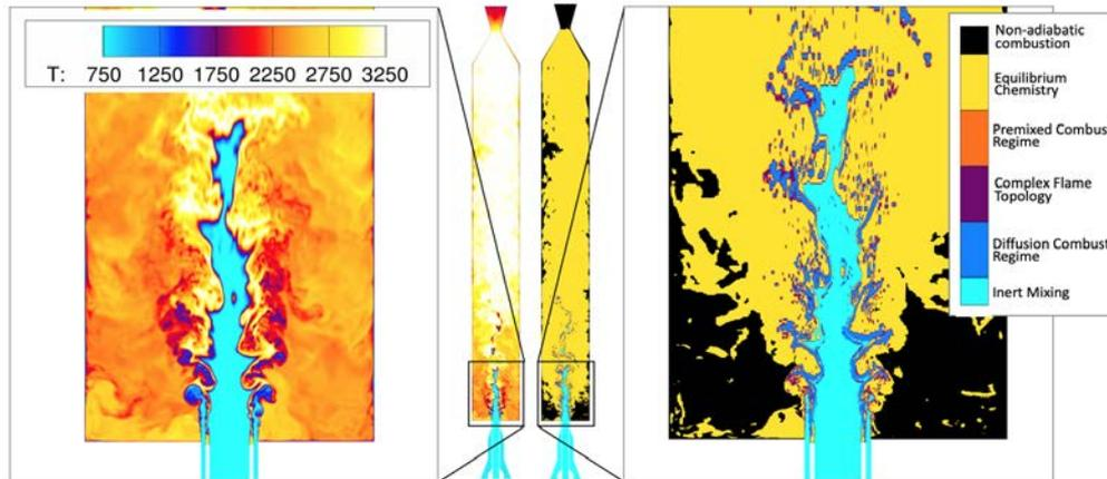
Figure 3: Combustion-mode analysis in a rocket injector.
