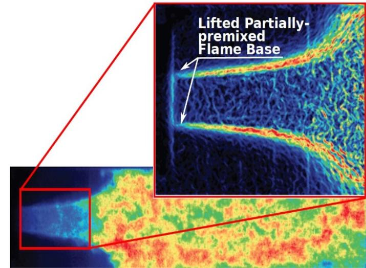
Lifted and partially-premixed flame base in LOX/GCH<sub>4</sub> supercritical combustion
