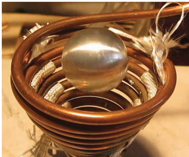
Figure 1: Levitation Melting using a copper coil (Sassonker et al. 2019)
