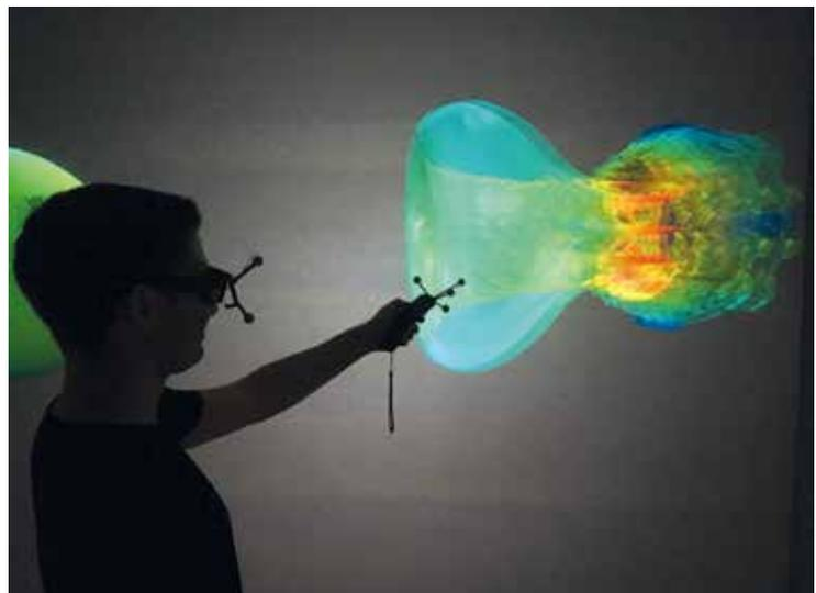
Shock-bubble interaction of an air-helium interface: 3D visualization of the late stage interface deformation at LRZ.
