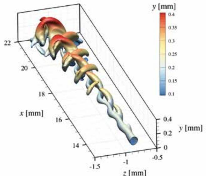
Vortical structures and breakdown downstream of a roughness patch for re-entry condition
