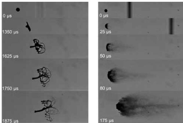
Shock-induced droplet break-up: bag-stamen type (left) and catastrophic type (right) for single water droplets ( $d=1\text{mm}$ ) with Weber numbers of 33 and 1310, respectively.
