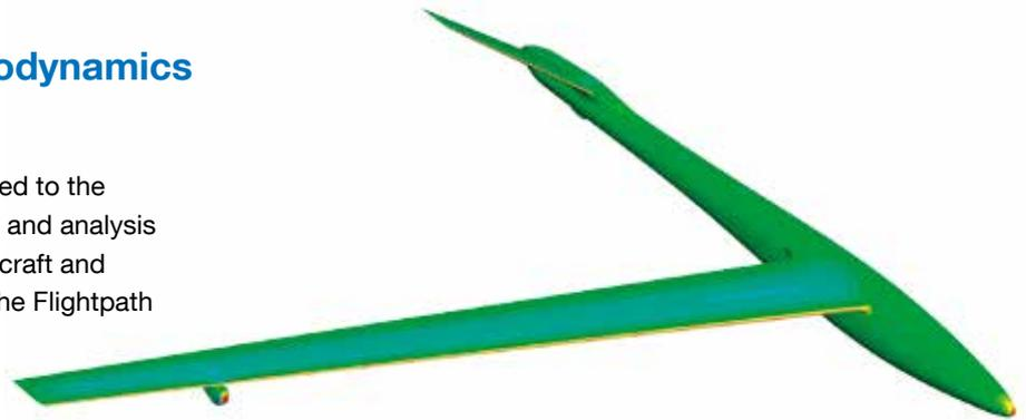
*Colored surface pressure distribution at FLEXOP flutter suppression demonstrator configuration.*
