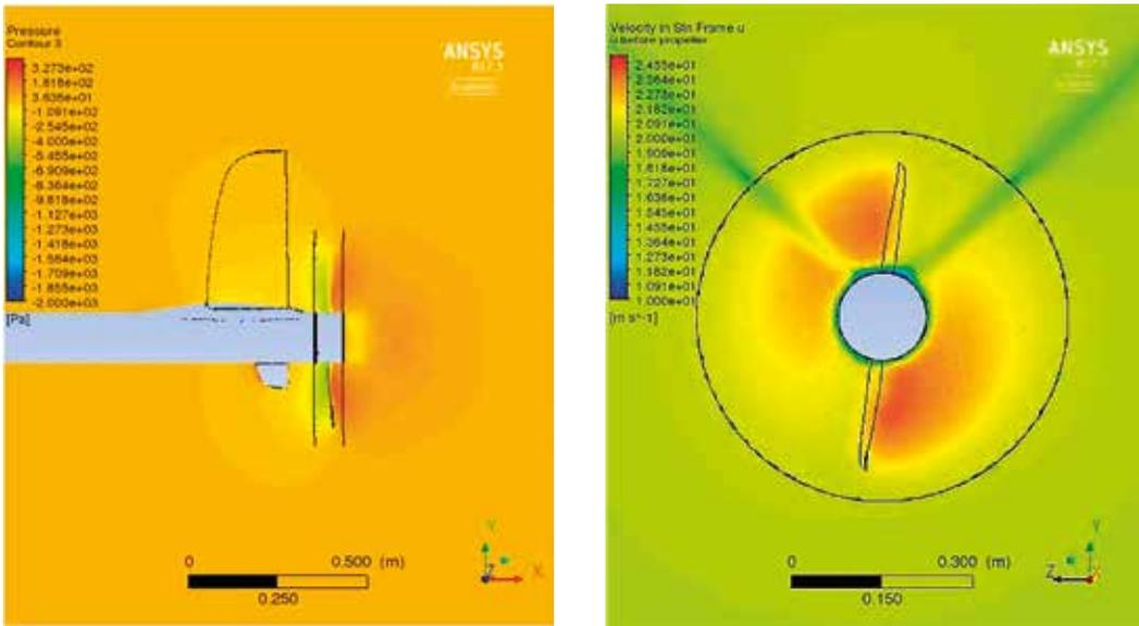
Figure 3: Left: Side-view of instantaneous static pressure in the tail section of the IMPULLS UAV equipped with a V-tail (empennage) and a two-bladed pusher propeller. Right: Magnitude of velocity in a cross-section between tail fins and propeller. Source: Peng Liu, Master's thesis, SBA, TUM 2018
