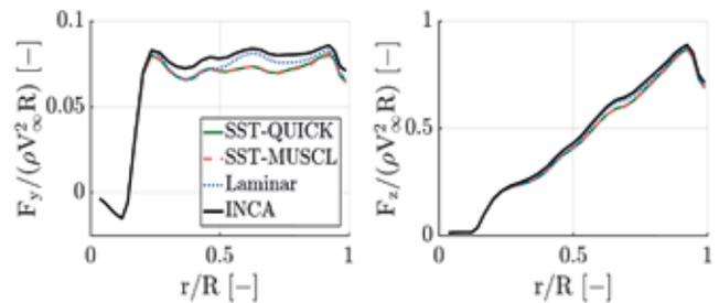
Figure 1: Tangential (left) and normal (right) component of the blade force along the radial extension of the blade for different turbulence models. From: Andrea Martinez-Garcia, term paper at SBA, TUM, 2018
