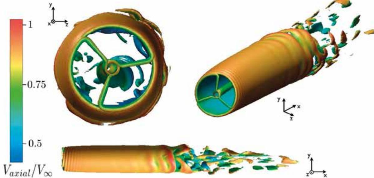
Figure 2: Isosurfaces of the axial component of the velocity in a wind turbine wake modelled in FLUENT with the ALM method. From: A. Martinez-Garcia, term paper, 2018
