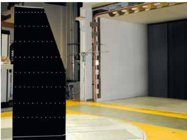
*Test bed of an elasto-flexible membrane wing configuration mounted in the test section of wind tunnel A.*
