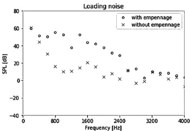
Figure 4: Comparison of loading noise in the far field at an observer position 45 degree off the axis from the pusher propeller with and without the empennage. Source: Peng Liu, Master's thesis, SBA, TUM 2018.
