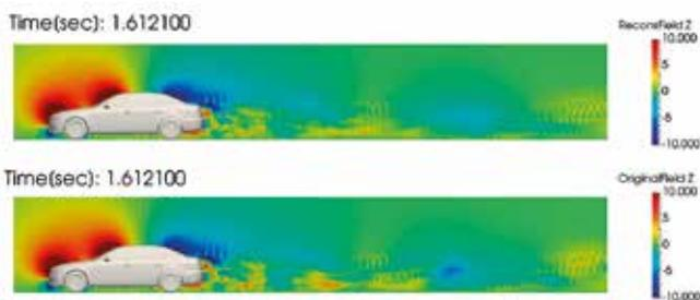
A snapshot of the instantaneous vertical velocity on the  $x$ - $z$ -plane at  $y=0.2m$  from the reconstructed field (above) and the original field (below).
