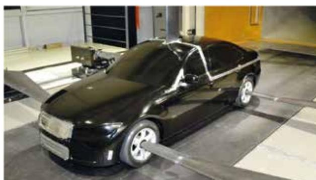
40% scale *DrivAer* model (notchback configuration) in wind channel A
