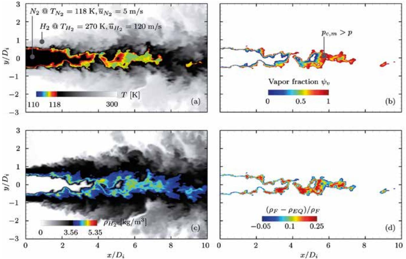
Instantaneous snapshots of a nitrogen jet in hydrogen: (a) temperature, (b) vapor fraction on a molar basis, (c) hydrogen density and (d) relative difference in density.
