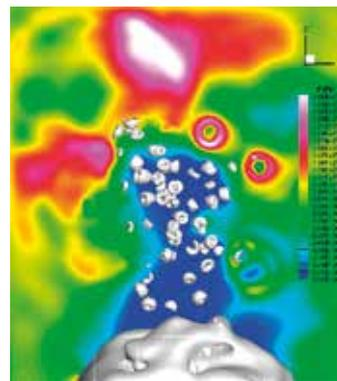
*Collapsed and partially rebounded vapor bubbles and vapor pattern located at a solid surface (bottom). The colors indicate the shock-wave intensity due to prior collapse processes.*
