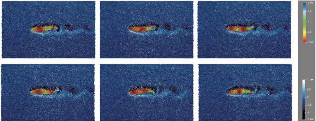
The sequence of results (ordered left to right and top to bottom) shows an SPH simulation of a tethered fish flapping in a stream with a Reynolds number of 1,000. An inextensible rope is connected to the left boundary. The color presents velocity magnitude of the fish body and vorticity in flow.
