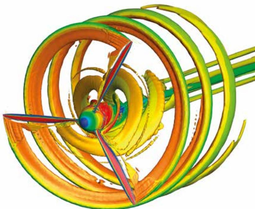
Computed (left) and measured (Stereo-PIV measurements for inhomogeneous inflow, right) propeller flow field.
