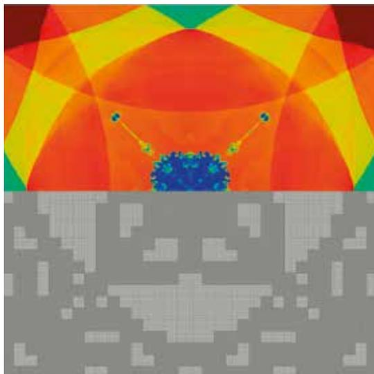
High-resolution simulation of an implosion problem: visualization of the pressure field and instantaneous grid representation showing the local refinement regions.
