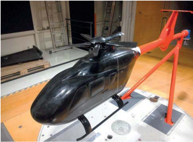
Model of BLUECOPTER configuration mounted in the test section of wind tunnel A.
