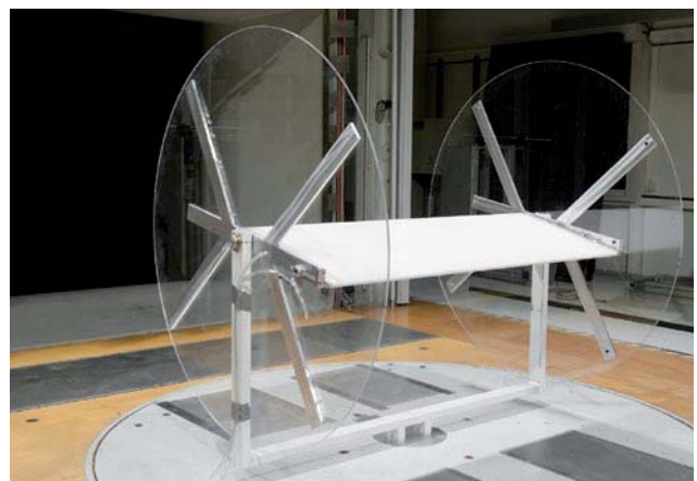
Test bed of an elasto-flexible membrane wing configuration mounted in the test section of wind tunnel A
