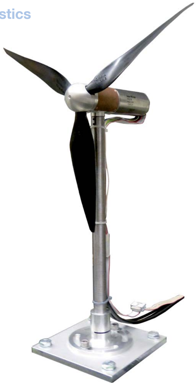
Figure 3: Model-scale wind turbine for the experimental investigation of the wake evolution over rough terrain in the atmospheric boundary layer wind tunnel of the Chair of Aerodynamics and Fluid Mechanics. The rotor diameter is about 450 mm.
