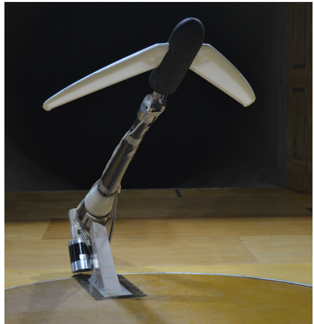
Figure 3: Wind tunnel model of a generic wing planform morphing configuration featuring an elasto-flexible lifting surface mounted in test section of wind tunnel A (MEMWing project)
